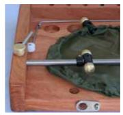
Insert the brass cam into the 15 mm hole on top of the left side of the base with the lever to the right.
