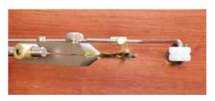
The small thumb screw at the point of articulation can be loosened and the distance from the bobbin to the hook adjusted to suit your needs.
